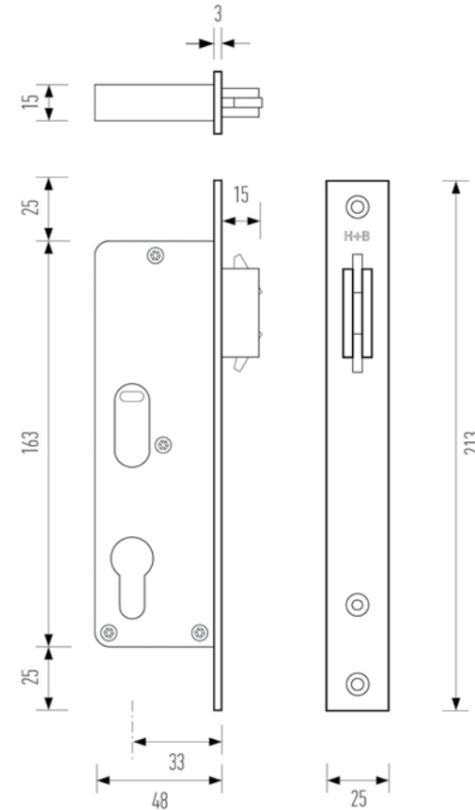
The Halliday + Baillie HB 640 sliding door lock set series allows several snib and key lock functions for sliding doors. Sliding the snib on either side operates the bolt unless a cylinder is engaged. A cylinder will lock the snib; the key does not operate the bolt.
