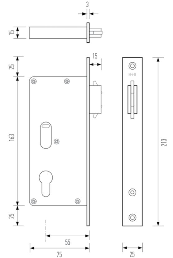
The Halliday + Baillie HB 630 sliding door lock set series function like the HB 640 series, but with a wider backset of 55mm.
