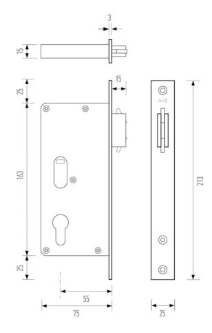
The Halliday + Baillie HB 630 sliding door lock set series function like the HB 640 series, but with a wider backset of 55mm.
