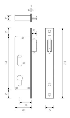
The Halliday + Baillie HB 640 sliding door lock set series allows several snib and key lock functions for sliding doors. Sliding the snib on either side operates the bolt unless a cylinder is engaged. A cylinder will lock the snib; the key does not operate the bolt.
