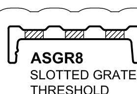
ASGR8 SLOTTED GRATE THRESHOLD Mass. 0.364 Kg/m Anod. Per. 105 Paint Per. 100 PREPUNCHED AND CLEAR ANODISED
