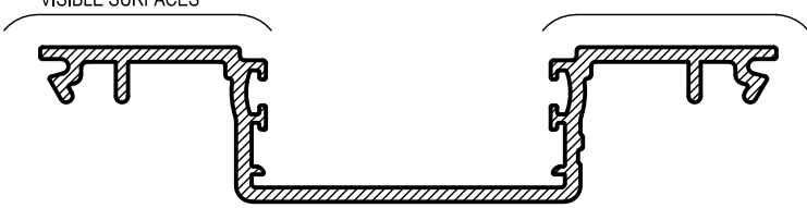
ECO204 101.6mm DG POCKET INFILL Mass. 0.741 Kg/m Anod. Per. 320 Paint Per. 180 Ixx = 193.60 x 10 3 mm 4 Iyy = 142.04 x 10 3 mm 4
