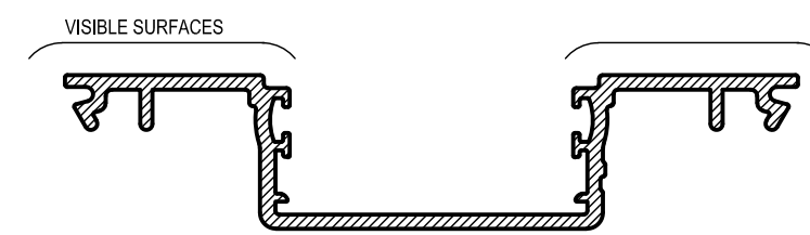
ECO204 101.6mm DG POCKET INFILL Mass. 0.741 Kg/m Anod. Per. 320 Paint Per. 180 Ixx = 193.60 x 10 3 mm 4 Iyy = 142.04 x 10 3 mm 4
