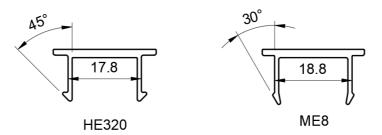
As part of the ongoing transition to the 19mm pocket. The Hawksbury MFE5 Jamb has now be upgraded to suit ME8 pocket filler and ME4 glazing adaptor, and will be known as MFE55.
