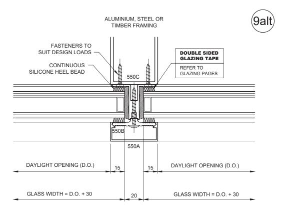
NOTE: SCREW SIZE AND QUANTITY TO BE CONFIRMED BY ENGINEER
