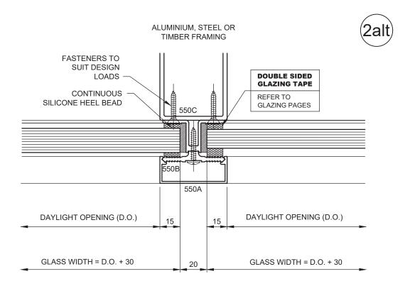
NOTE: SCREW SIZE AND QUANTITY TO BE CONFIRMED BY ENGINEER
