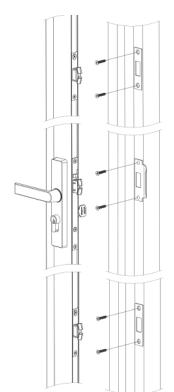
Line up the strikers and secure with 25mm CSK screws.
