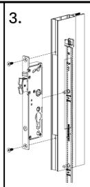
With the lock bolt extended and deadlocked, insert the centre lock into the cutout, ensuring the actuating bar's locating lug engages. Secure the lock with two 12mm CSK screws.
