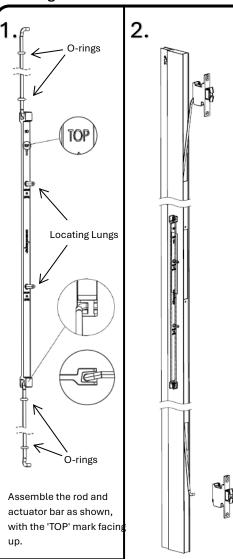
Starting with the bottom rod, insert the rod assembly through the top cut-out and slide it into the door section.
