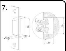
Close the door and mark the jamb at the centre of the main hook bolt and multipoint locks. Then cut a 20x35mm bolt recess from the centre of the mark.
