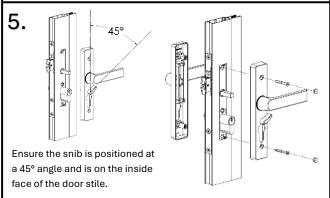
Secure the furniture plates as indicated above, using 25mm CSK screws, then insert the concealed fixing screw caps.
