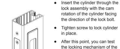
To test the cylinder, the anticrash pin must be held down and snib thrown to activate the bolt. Cylinder can now be turned to lock bolt.
