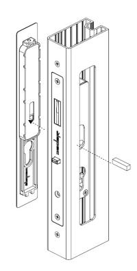
If the furniture plate with snib is on the deep lockbar recess side, place the E-clip on groove **A** on the spindle.
